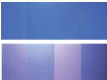
Lighting conditions can cause objects to look the same even when their colors are different, a condition known as metamerism. The image shows four blue patches under white LED (top) and quartz-halogen lighting (bottom). Source: Edmund Optics
